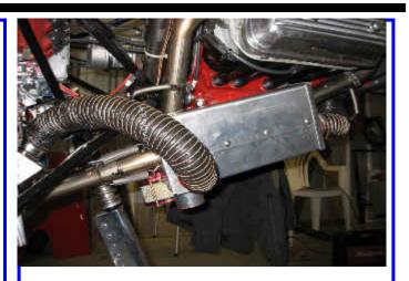
The front tube enters at the bottom of the box and is directed by a 45 degree baffle, just inside, to the top of the box, where the pipe is located. The exit tube comes out the bottom side at the rear and goes to the heat valve on the fire wall. The tubing is all 2 inches. The tube that exits on the bottom is
