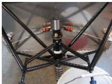
I had to cut the top of the gear tube off to get the box in at all, and could not move it to the right due to the strut. The box shown is built for, and contains an Odyssey dry cell battery.
