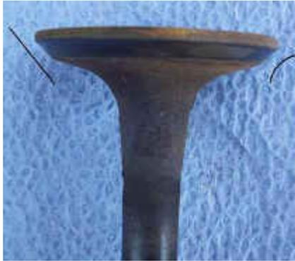
side) next to the tuliped area. I've highlighted the valve face discrepancy.
