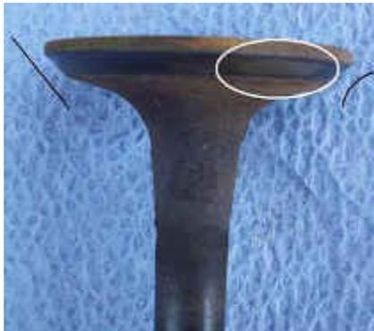
(oval), the valve wobbles and doesn't seat properly. This causes "tulip" wearing on the valve face. Valve erosion starts due to lack of seat contact cooling and exhaust gas blowby.
