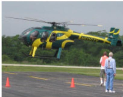
rotor, just a large tubular tail boom that housed a fan that forced air thru louvers in side of the boom at the tail. The boom also had slots running the
