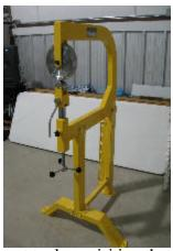
This is the latest tool acquisition the Chapter has made. The English Wheel, donated to the Chapter by Barry Logan, is used to make compound curves in any malleable metal.
