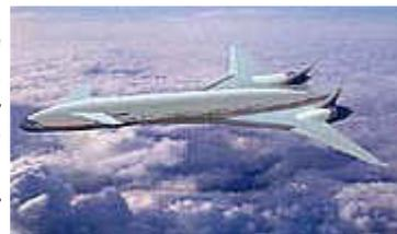
Mulally said the airplane will be able to fly 20% faster than existing jet models, at Mach 0.95. That is 95% the speed of sound or roughly 740 miles per hour. It could cut 3 hours off a flight from the West Coast to Europe, he said.
